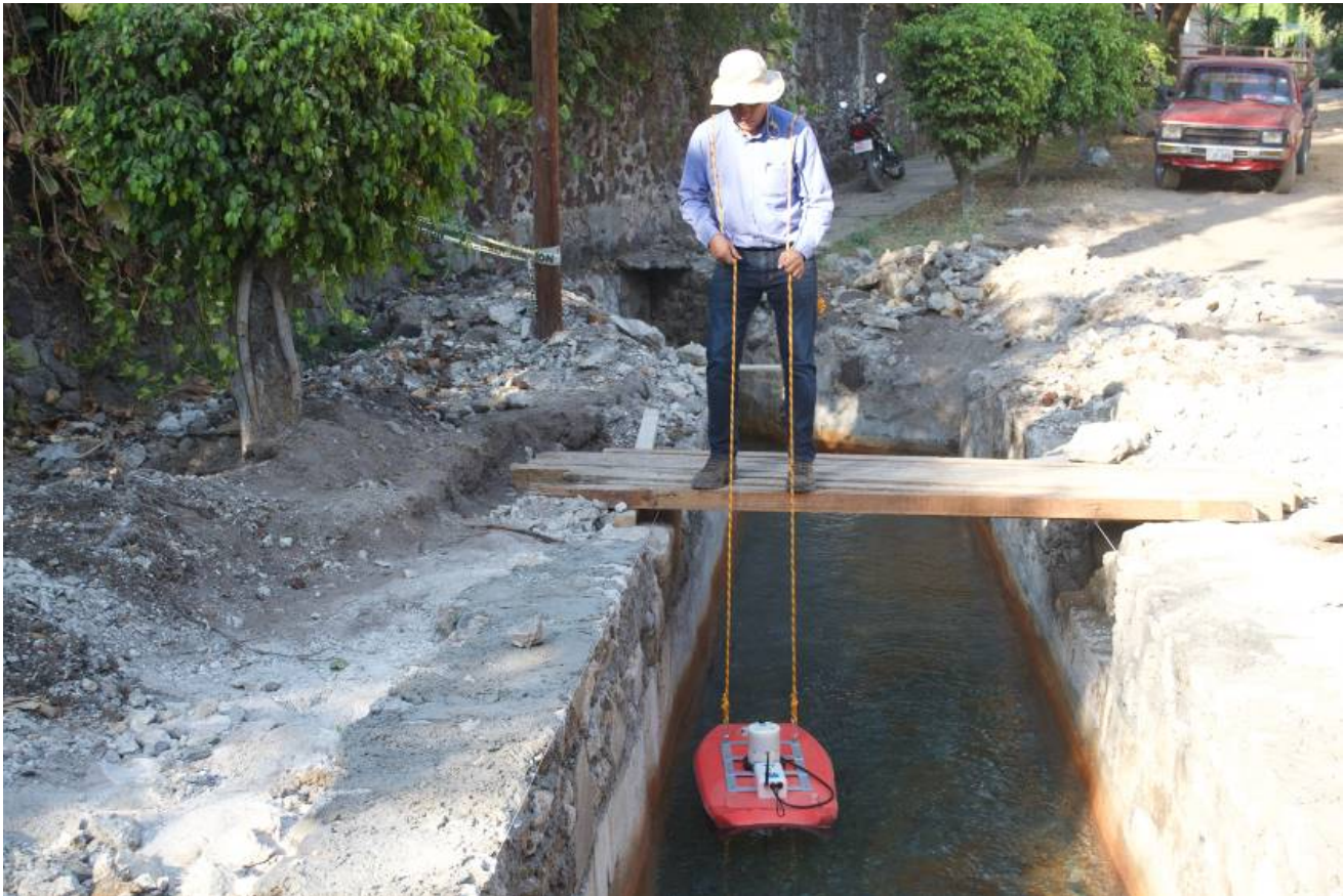
Figura 6.16 Aforo del manantial “Santa Rosa”.
